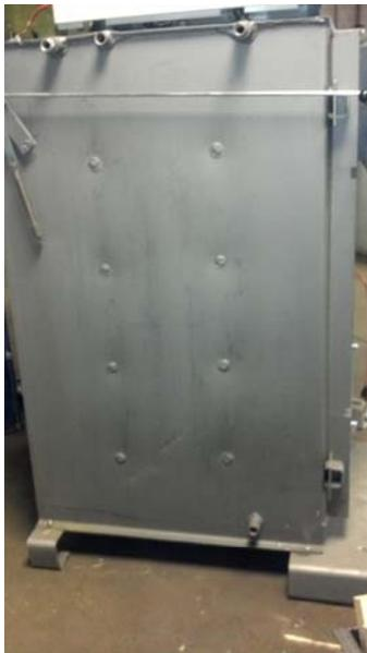
You will also note the ‘bulging’ of the sides of the European boiler that occurred during factory pressure testing. In addition to the correct amount of ‘stays’ to hold the boiler together, Econoburn uses 1/4” SA-36 boiler plate. Conversion of the European-built 4mm yields just over 1/8” steel thickness.
